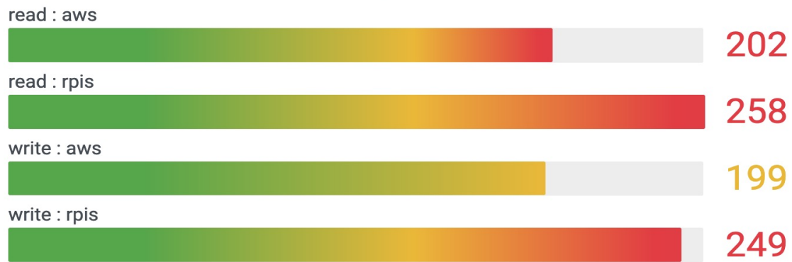
Figure 19 - The Deployment Effect on Read/Write Operations latency RPIS vs AWS – Type:Stoch, Leaders 5, Followers 2
